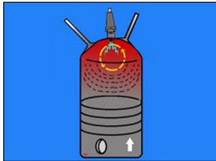
Figure 3. Tumble Flow Induction in single spark ignition engine
